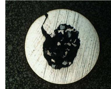
Section of seamed flux cored wire
