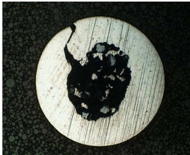
Section of seamed flux cored wire
