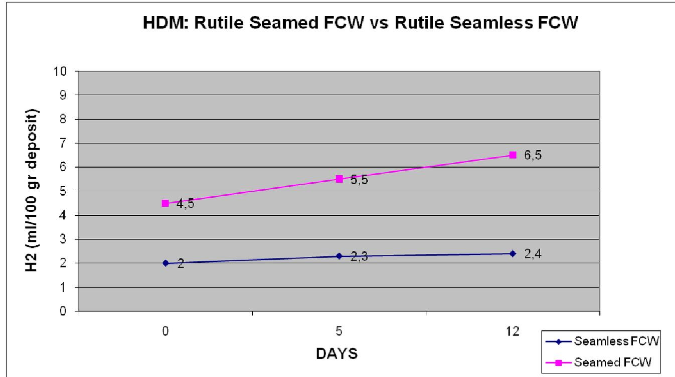
WELDING CONDITIONS: 25V – 250A – STICK-OUT: 17 mm - GAS: M21
