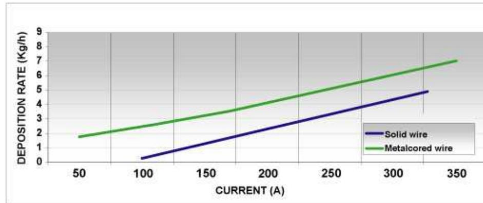
Difference in deposition rate between solid wires and flux cored wire
