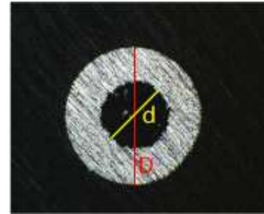
Cross section seamless flux cored wire
