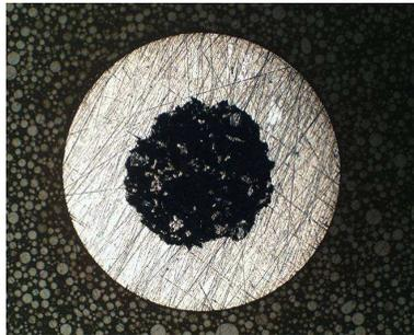
Section of seamless flux cored wire
