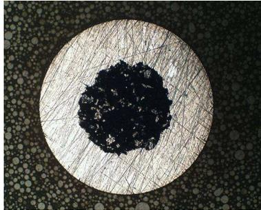
Section of seamless flux cored wire
